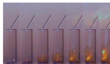
Figure 2. Hypergolic testing of azo substrate 4 with MMH.
